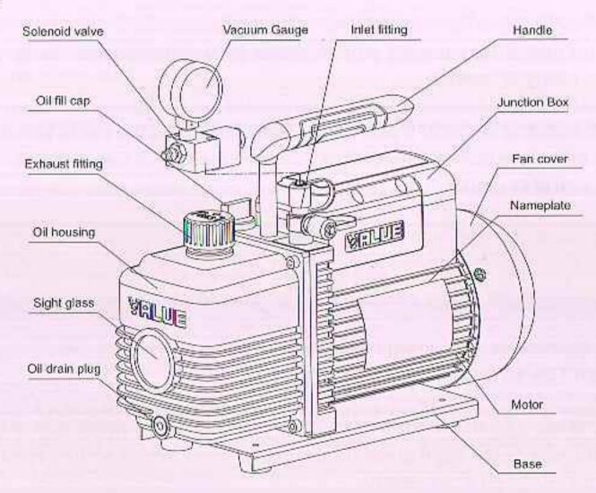
Remark: Only new refrigerant series are assembled with solenoid valve and vacuum gauge
